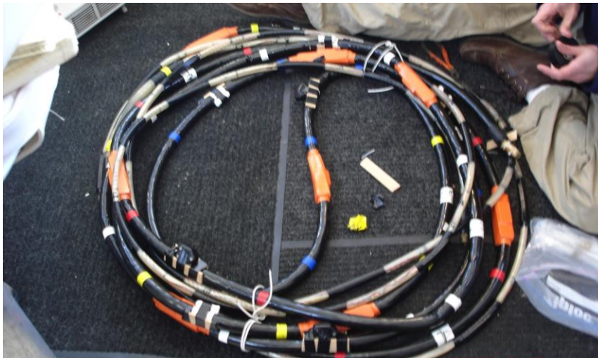
Figure 4. The OASIS Towed Array wrapped and coiled on the deck prior to deployment.
